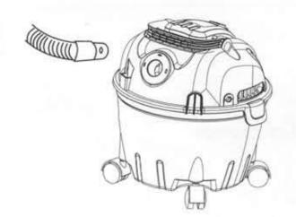
inserting thehose into the exhaust hole: turning on the switch, it can blow off the dust
