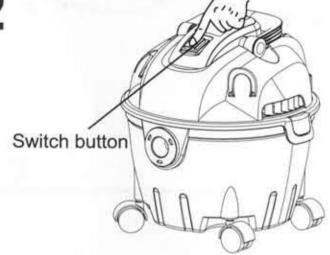
Press the switch button to turn on/off the cleaner.
