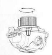
Twist the locking knob with a anti-clockwise force, take off the filters
