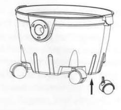
Install castor wheels into the hole on the base.
