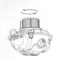
Twist the locking knob with a anti-clockwise force, take off the filters
