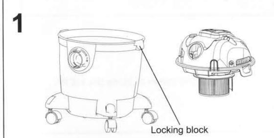
Release the lock block to open the up housing
