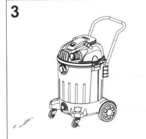
Put back the up housing, and fasten the locking block
