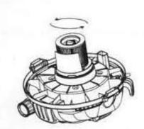
Twist the locking knob with a anti-clockwise force, take off the filters
