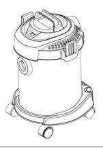
Put back the up housing, and fasten the locking block
