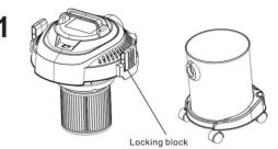
Release the lock block to open the up housing
