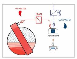
The Barista can adjust the temperature individually and control it **directly by the display:**
