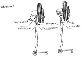
a.Refer to diagram 3. Plug the four-pin plug of power cord into four-pin socket on the lower part of the stand pole. And locate them into the stand pole after connection.
