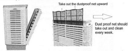
Pull out the power supply power plug, screwing out the screws from the louver by electric drill. Holding the top of louver and pull out (with a bit pull upward), remove the cooling pads kits and wash them by high pressure water gun, until the dirt complete be washed out.
